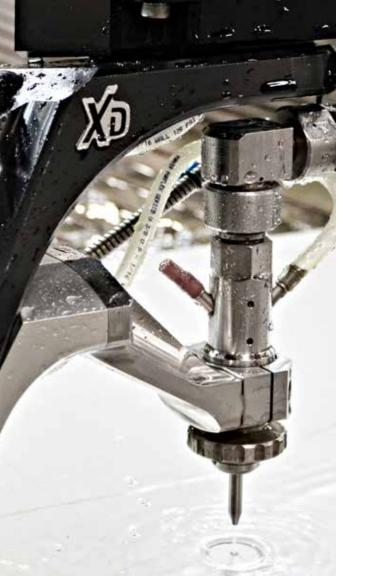
(+/- 0.03 to 0.08mm). The technology allows the machine to move very fast, create a taper and stream lag, and then compensate for it automatically by tilting the head by up to 10 degrees.
