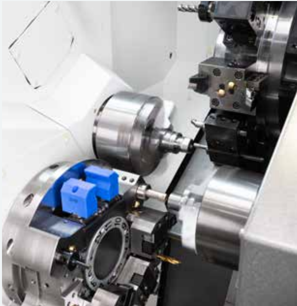
Lower Turret Max. 9 Stations without Milling function + Unloading Gripper
