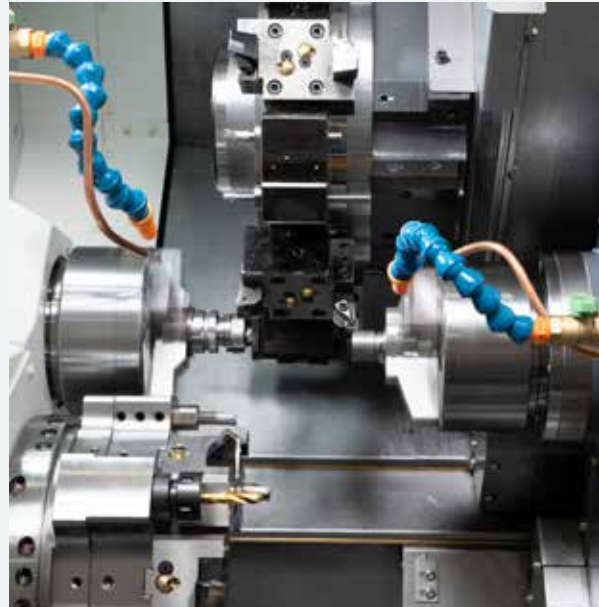
Superimposed cycle is simultaneous machining through overlapping control between Main spindle and Sub-spindle.
