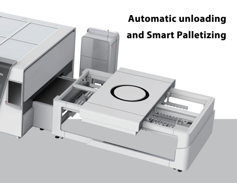
Adopt belt conveyor and adjustable width-limiting device. After processing, sheets will be automatically transmitted to unloading device, and palletized by lifting device according to material width. No manual sorting will be needed after processing, improving efficiency and saving labor.
