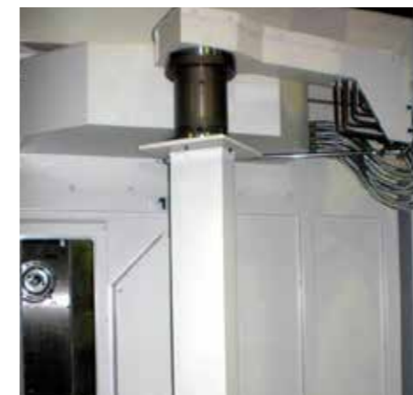
Example of the use of 6-port rotary joint (HM400/500S, HM5100/6000S, HM6300/HM8000S, HM1000/1250S)
