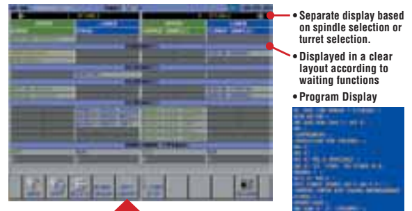
Waiting function is easily input with the push of a button
