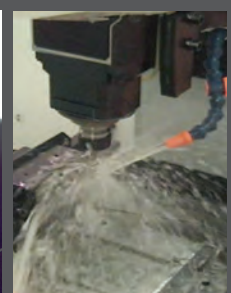
High pressure coolant system
