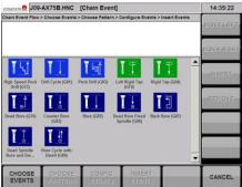
Conversational Event Based Programming allows making part programs by simply choosing machining events and configuring its parameters, without having to write G-Code.
