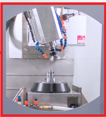
Single or twin spindles available on larger grinding platforms: HSK quick change tooling, ceramic bearings, liquid cooled for better process consistency and control
