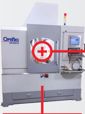
Rigid cast iron base for excellent stability (e Series and SXL 500 machines)
