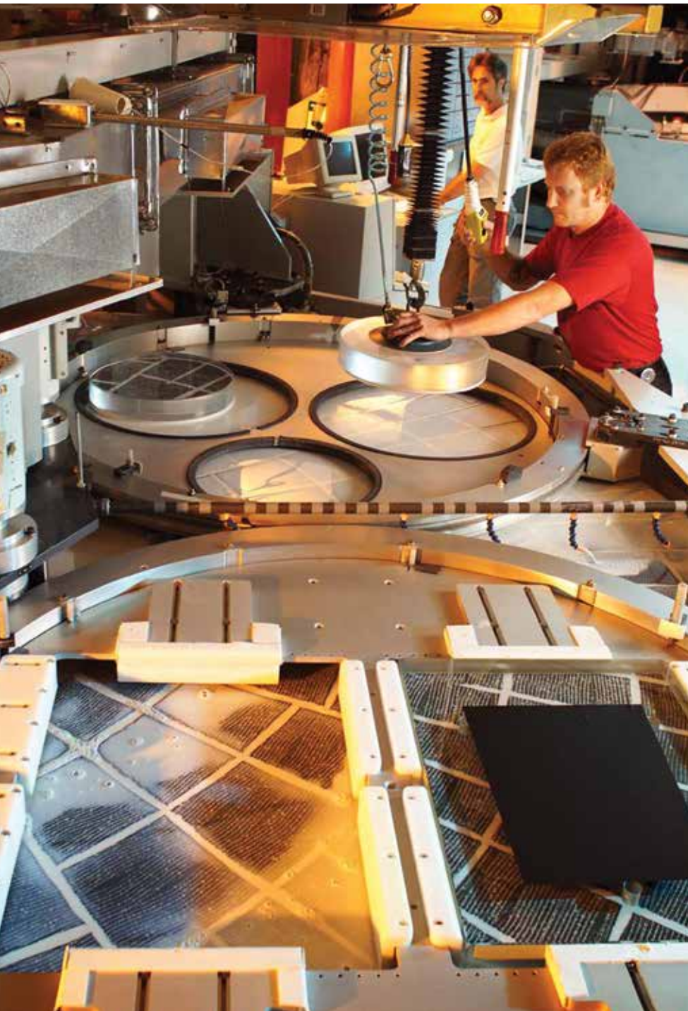
Polishing large optical flats as part of the fabrication process.
