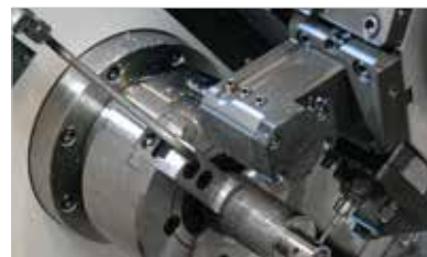
Chuck Air Blow (Upper Chuck)
